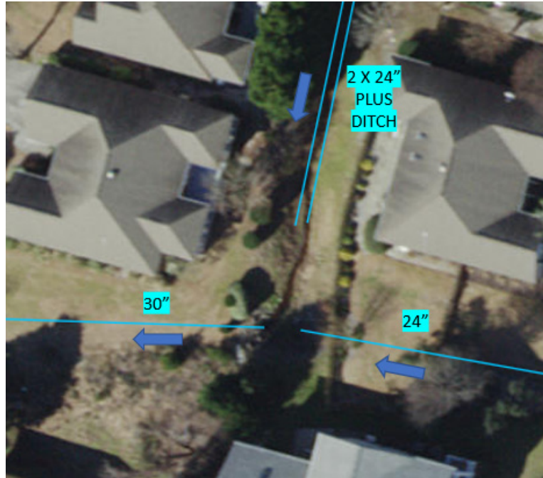
Figure H: A Choke Point Between N 5 th Ave and Settler's Ln
