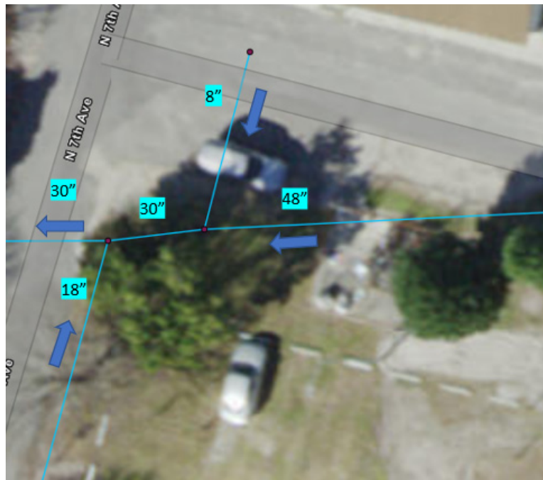
Figure F: A Choke Point Behind the Fire Station on K Ave
